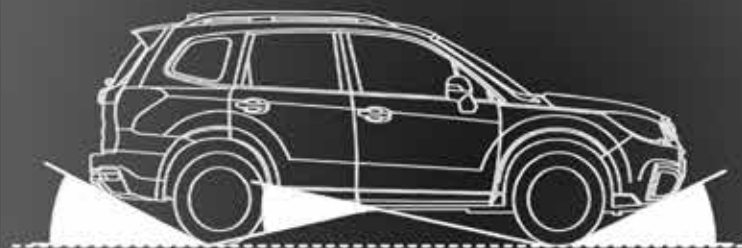
Departure Angle Break-over Angle* Approach Angle
